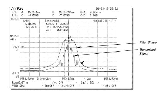
It can be seen from the diagram above that as the channel spacing gets closer, the shape of the filter becomes more critical. *Extracting a 10-Gbps signal when channels are spaced at 50-GHz, is technically difficult.*
